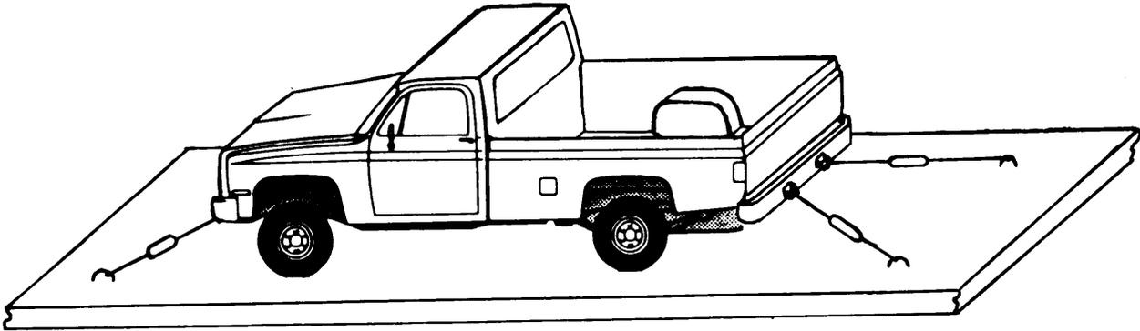
*Figure 6-4. Typical tiedown of CUCV in RORO vessel.*
