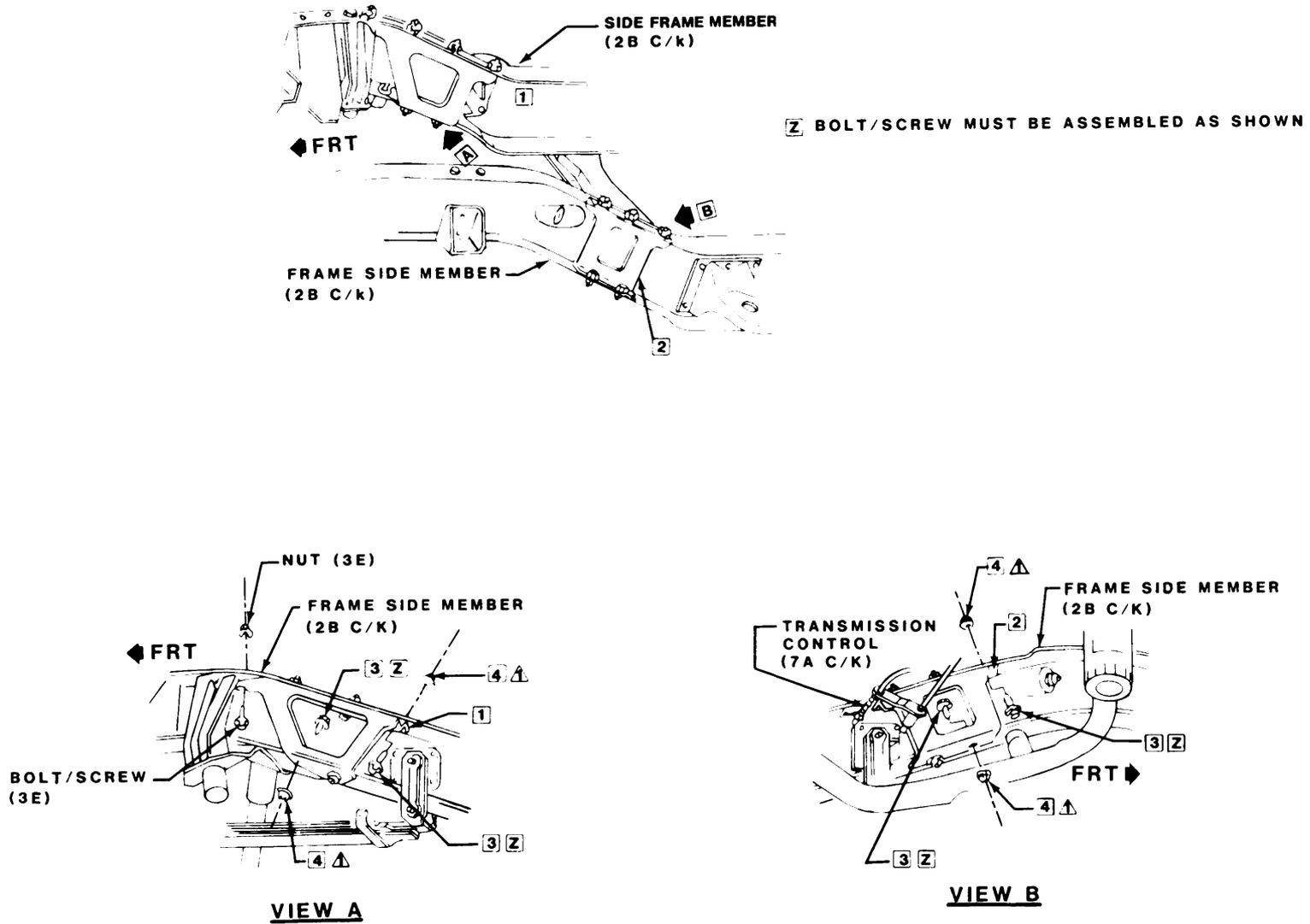
Figure 2-8. Frame reinforcement bracket, front.
