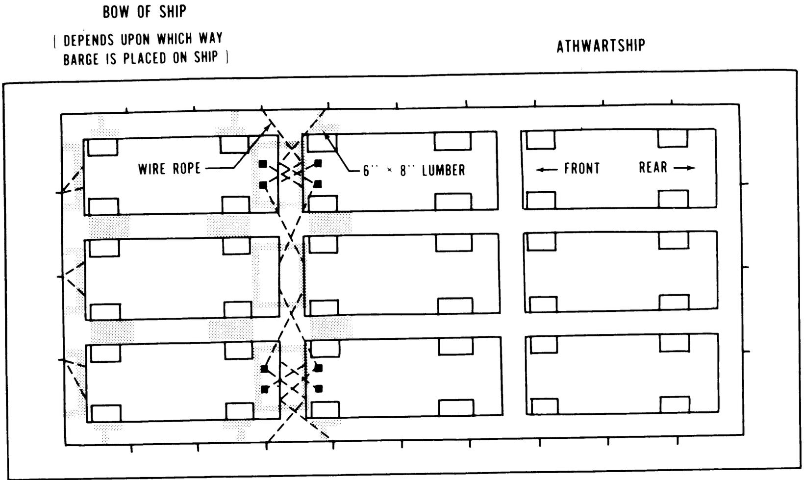
BLOCKED AND BRACED WITH WAY 6" x 8" LUMBER.
