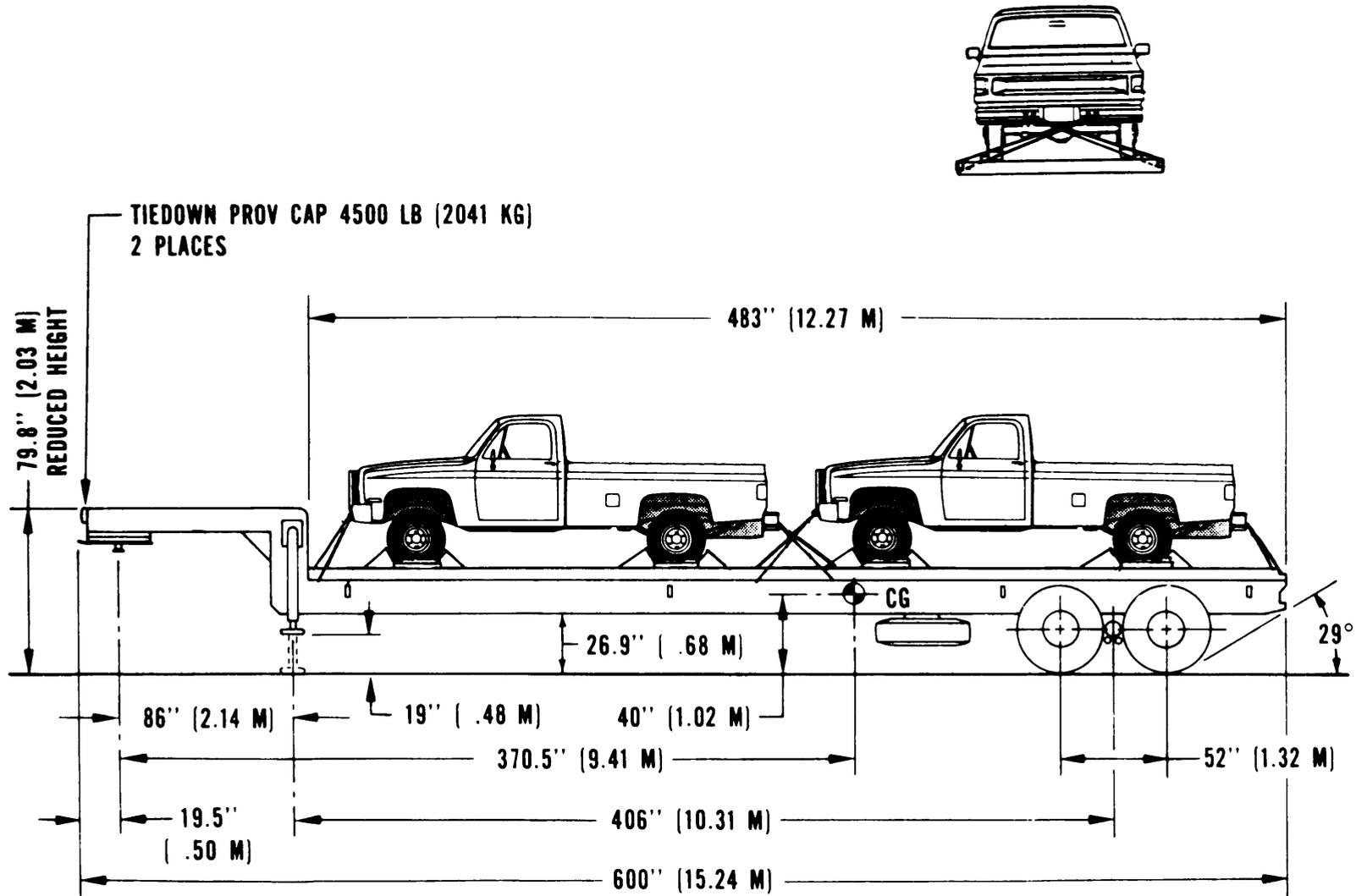
Figure 5-1. Tiedown of CUCV on a semitrailer.
