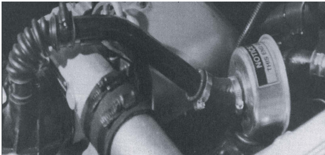
Figure 16-18, Crank Case Depression Regulator Valve
