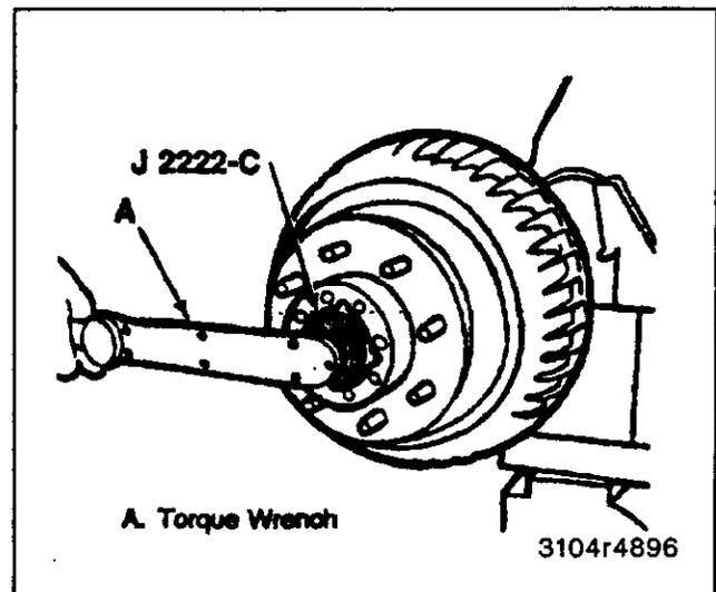
**Figure 35—Tightening the Adjusting Nut**
