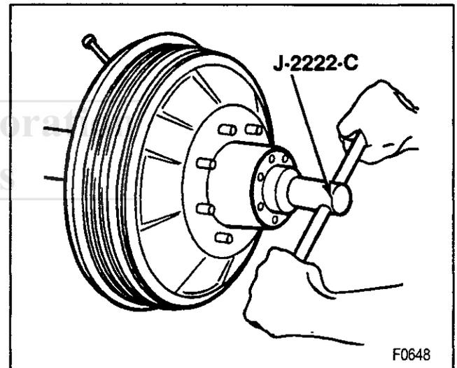
Figure 22—Removing or Installing Bearing Adjusting Nut
