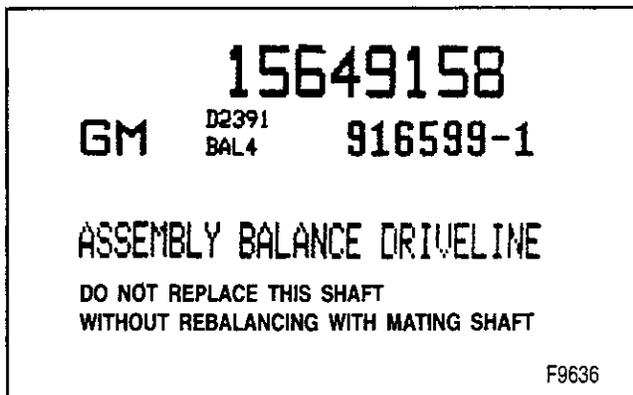
Figure 12—System Balanced Propeller Shaft Assembly Notice
