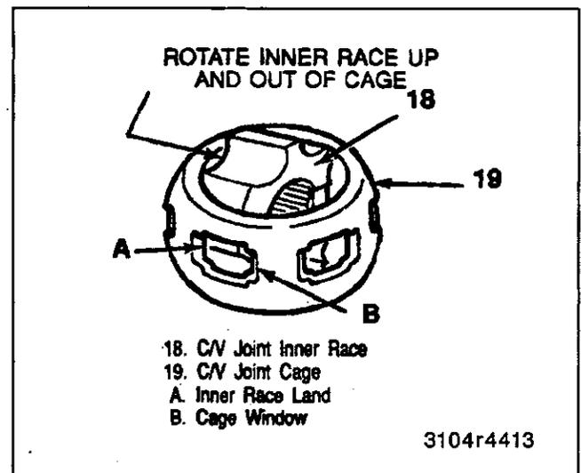
Figure 18—Separating Inner Race and Cage
