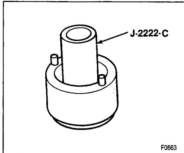
Figure 25—Wheel Bearing Nut Wrench
